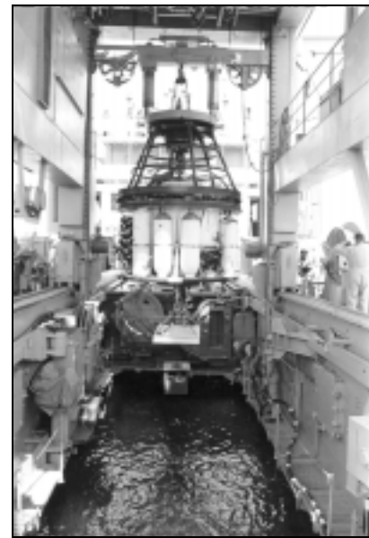
Figure 1-20. PTC Handling System, Elk River .
